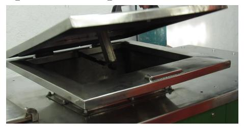
Food waste is fed into the inbuilt shredder.
